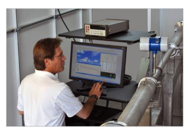
Fox Thermal's Calibration Lab utilizes NIST-traceable equipment.
