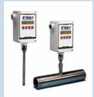
The Fox Model FT2 Thermal Gas Mass Flowmeter and Temperature Transmitter measures two important process variables with one rugged instrument. The Model FT2 measures gas flow rate in standard units without the need for temperature or pressure compensation. It provides isolated 4 to 20mA and pulse outputs for flow rate, and a 4 to 20mA output for process gas temperature. The pulse is normally used for totalization. [Learn More](#)
