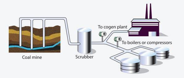
Methane recovery from coal mines can power equipment on-site.
