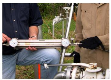
Sampling natural gas from the source is the best way to determine the gas composition.
