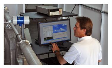
Calibration Technician performing an actual gas calibration in the flow laboratory.
